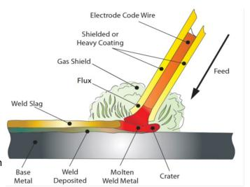
When the electrode is moved along the work piece at the correct speed the metal core deposits a
