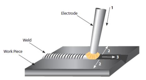
The operator can choose the manipulation of the electrode based on welding joint, welding position, electrode spec, welding current and operation skill etc.
