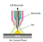
The ARC 400 range allows the tungsten to be in direct contact with the work piece with minimal current so as not to leave tungsten deposits. Once contact has been made the tungsten can then be lifted away 2-4mm from the work piece and the welding arc is then established.
