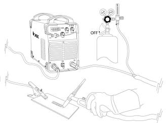
After connecting the welding leads as detailed you will need to switch the power switch on the back panel to "ON". Select Lift TIG by switching to TIG on the MMA/TIG welding mode switch. (Note, there is voltage output at both output terminals).
