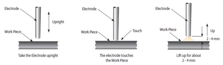
**Scratch technique** - Drag the electrode and scratch the work piece as if striking a match. Scratching the electrode may cause the arc to burn along the scratch path, so care should be taken to scratch in the weld zone. When the arc is struck adopt the correct welding position.
