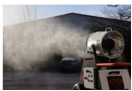
The CANNONMISTER is an answer to environmental dust and odour hazards. The CM10-HP will suppress fine airborne dust particles with its electric-powered fan blowing fine water droplets created by special misting nozzles. The dust cannon has a high-pressure water pump only using 2 litres per minute, which saves water and reduces flooding the site. Ideal for fine dust, odour control and disinfectant misting.
