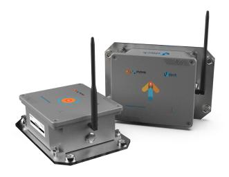
Deck is the only sensor on the market for measuring the dynamic oscillation amplitude with an accuracy of 0.01 mm. It also detects the temperature and vibration frequency of any structure. Perfect for continuous remote monitoring of dams, bridges, viaducts and buildings and for dynamic load tests. Wireless device with battery power and LoRaWAN transmission.
