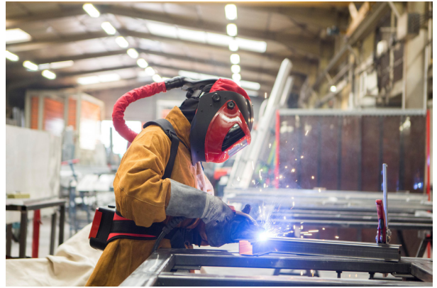
An example of personal fume extraction
