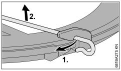
Disconnect wire rod from the transport guard.
