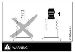
Arcing may occur if the adapter nut (1) is loose or missing. Working in an easily combustible or explosive atmosphere may cause a fire or an explosion. This can result result in serious injuries or damage to property.
