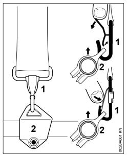
Press down the bar on the carabiner (1) and pull the carrying ring (2) out of the carabiner. 15 Starting / Stopping the Engine
