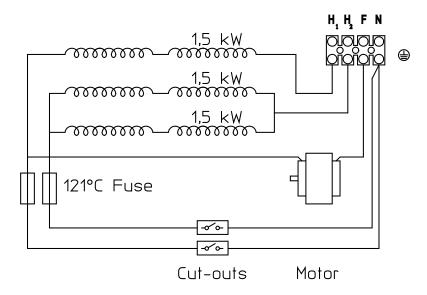
Circuit Diagram 4,5kW Heaters
