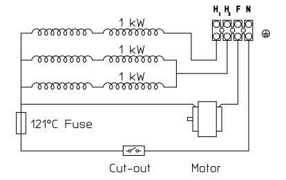
Circuit Diagram 3kW Heaters
