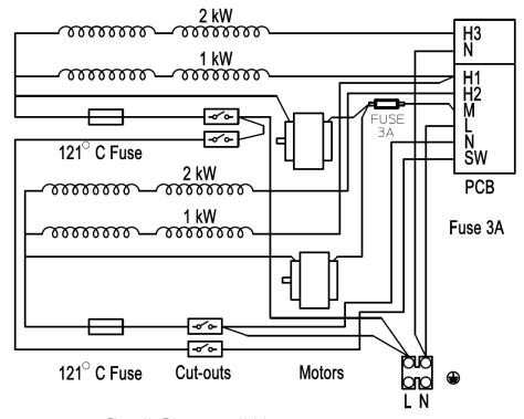
Circuit Diagram 6kW Heaters for Wireless Controls
