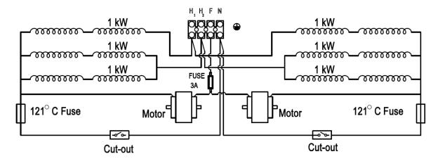
Circuit Diagram 6kW Heaters
