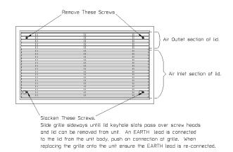
Fig.3 Grille fixings detail
