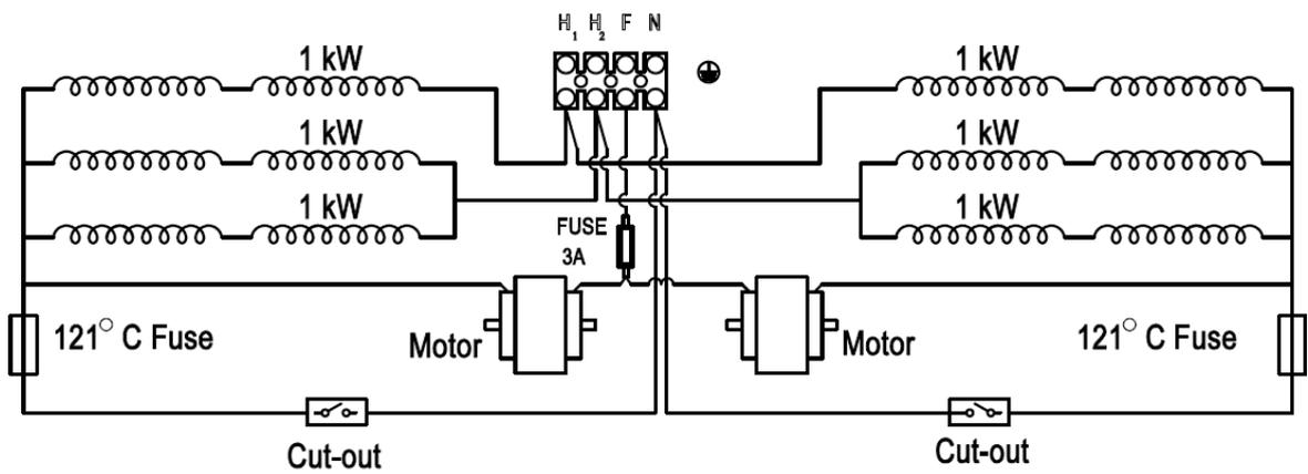
Circuit Diagram 6kW Heaters
