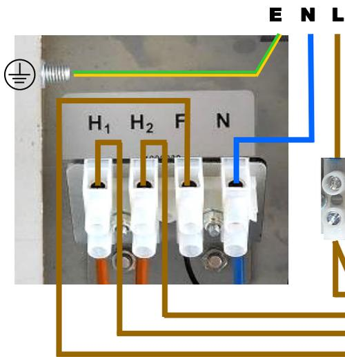
Fig.10 Remote switch terminal side view
