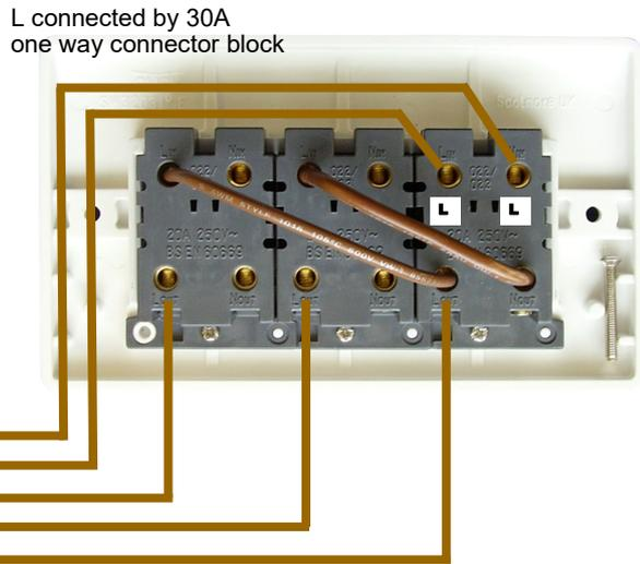
Fig.11 Mains supply via remote
