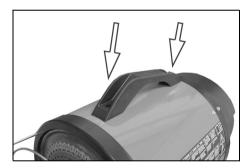
4. Fit the heatshield to the heater body using the screws supplied.
