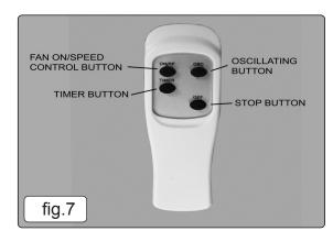
5.4.4. **TIMER BUTTON :-** Press to select working time, 1/2, 1, 2, 4, hours indicated by the LED lights on the fan control panel (ie. by adding the selected fig. displayed above LED.) **Note:** As the timer counts down the speed of the fan will reduce.
