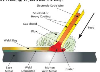
When the electrode is moved along the work piece at the correct speed the metal core deposits a uniformed layer called the weld bead.
