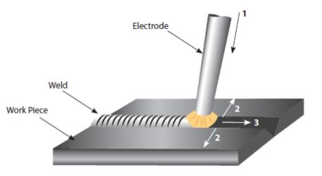
The operator can choose the manipulation of electrode based on welding joint, welding position, electrode spec, welding current and operation skill etc.
