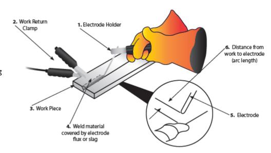
Welding current will flow in the circuit as soon as the electrode contacts the work piece. The welder should always ensure a good connection of the work clamp. The nearer the clamp is placed to the welding area the better.
