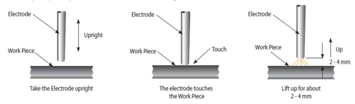
**Scratch technique** - Drag the electrode and scratch the work piece as if striking a match. Scratching the electrode may cause the arc to burn along the scratch path, so care should be taken to scratch in the weld zone. When the arc is struck adopt the correct welding position.
