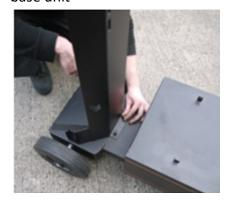
Place the power source on the base unit and locate the brackets on the base to the brackets on the base assembly. Use 4 x M5 screws to secure the power source to the base assembly.
