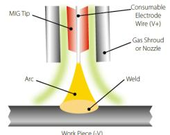
MIG welding was developed to help meet production demands of the war and post war economy which is an arc welding process in which a continuous solid wire electrode is fed through a MIG welding gun and into the weld pool, joining the two base materials together.
