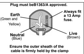
We strongly recommend that this machine is connected to the mains supply via a Residual Current Device (RCD).
