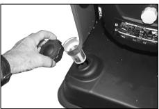
do not overfill. Use a funnel or can with a long filling spout.
