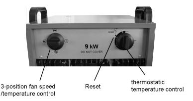
The thermal cutout may also operate if the heater is shut down without allowing to cool sufficiently. If subsequently, the heater fails to start, press the RESET using a suitable tool and try again.
