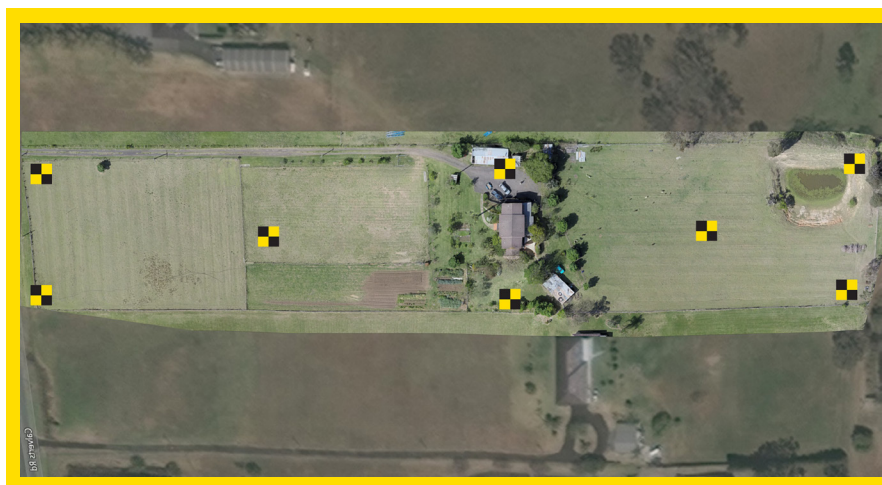
Figure 3 | Orchard Hills test site with recommended AeroPoints distribution
