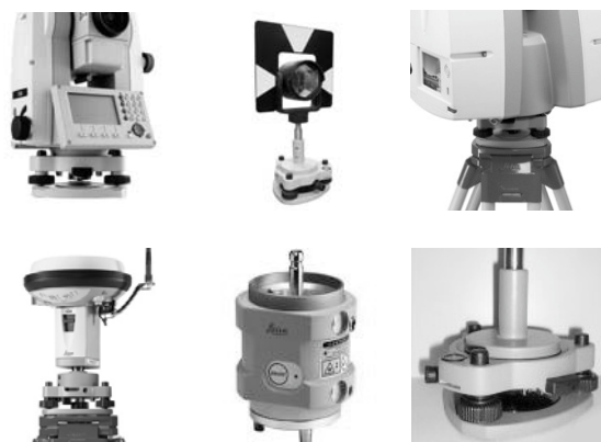
Figure 14 - Different devices requiring a tribrach in order to be used at all
