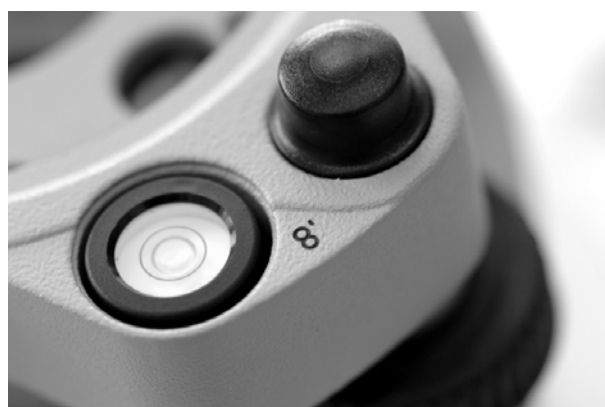
Figure 4 - Detail view of the GDF121 circular bubble
