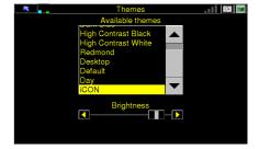
B When the brightness is set to max the backlight on the on-panel buttons is turned off.
