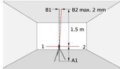
Set up the laser on its tripod o wall mount bracket near point A1 at a minimum distance of 1.5 m from point B1. The horizontal laser is aligned in direction 1. Mark the laser points A1 and B1 with a pin.
