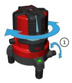
Turn adjustment knob (1) for fine adjustment of vertical laser lines.
