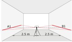
Set the instrument on a tripod half-way between two walls (A+B) that are approx. 5 m apart. Place the lock switch in the "Unlocked" position. Direct the instrument at wall A and switch on the instrument. Activate the horizontal laser line or laser point and mark the position of the line or the point on wall (A1). Rotate the instrument by 180° and mark the horizontal laser line or the laser point in exactly the same way on wall (B1).
