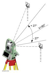
Measure to measure and to continue to the next screen. Motorised instruments change automatically to the other face.
