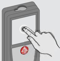
Tap on the display to open an on-screen button or to make a selection. Tapping on the icon in the middle of the bottom line activates the distance measurement or triggers the camera.
