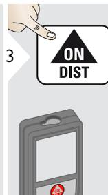
It is absolutely necessary to aim with the laser perpendicular to the object.
