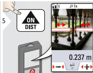
Select arrows with the cursor keys or by tapping on the display and adjust with softkeys. Corresponding diameter is calculated.
