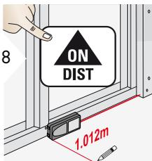
Move device slowly along the stake-out line. The distance to the next stake out point is displayed.
