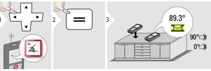
Inclination is permanently displayed. Instrument beeps at 0° and 90°. Ideal for horizontal or vertical adjustments.
