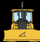
Total Station Control
