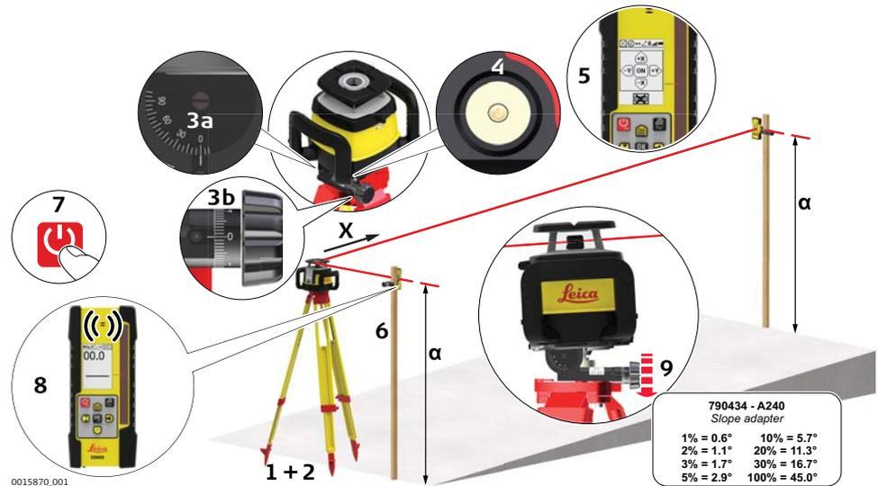
1. Set up the Rugby and the slope adapter on a tripod.
