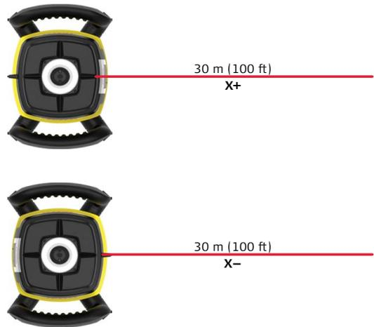
2. Align the first axis so that it is square to a wall. Allow the Rugby to self-level completely (approximately 1 minute after the Rugby begins to rotate).
