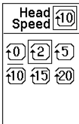
The currently active option is underlined. Press the OK/Grade button to select an icon. To navigate to the second menu page, press Right arrow/Volume button until page two is displayed.
