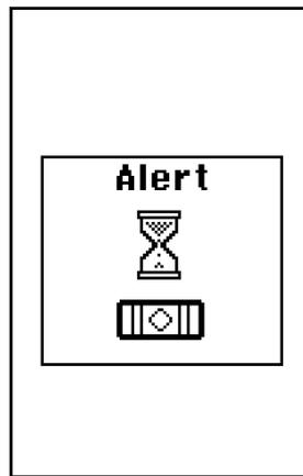
When the Rugby is re-levelling, the Temperature check wait screen is displayed. Wait until the process is finished before using the laser again. The Status LED flashes on the Rugby to indicate normal levelling.
