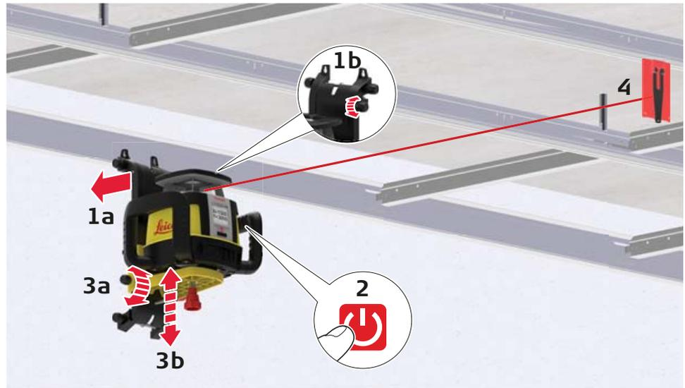
1. After mounting the first strip of ceiling trim at the desired height (centre position of the ceiling target) below, attach the Smart Adapter and laser to the trim. Tighten the locking knobs on the top of the Smart Adapter.
