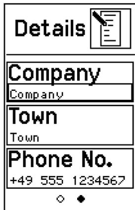
You can enter 3 lines of text with up to 15 characters per line. The fields are specified as:
