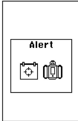
When the number of planned hours is reached, the calibration alert is displayed for 8 seconds. After calibrating the Rugby, the calibration alert hours are automatically reset. Changing or disabling the calibration alert is only possible by accessing the menu option "Calibration alert function".
