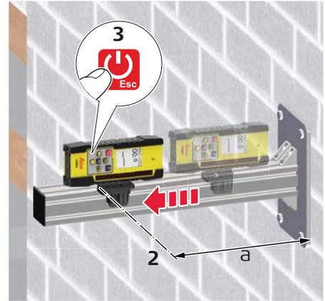
1. Mount the Combo to the receiver bracket using the 90 ° adapter.
