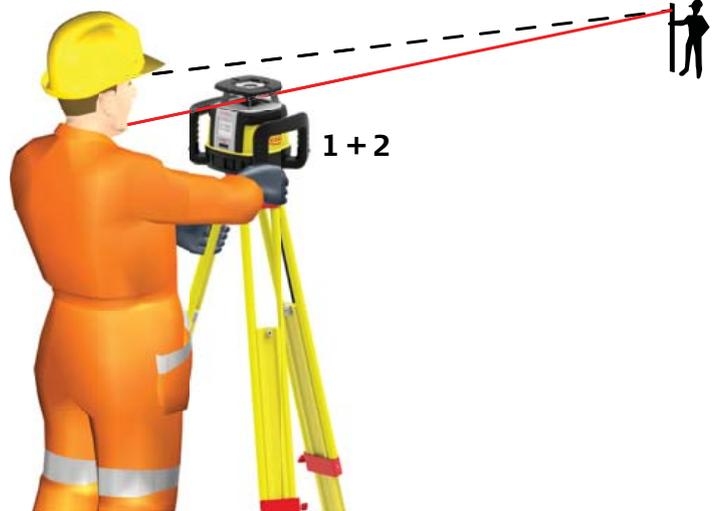
1. Set up the Rugby on a tripod.
