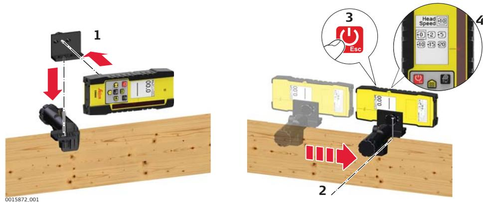
1. Mount the Combo to the Combo bracket using the 90 ° adapter.
