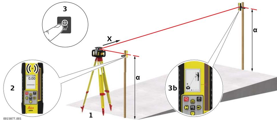
1. Ensure that the grade value is set to zero. Set up the Rugby at the base of a slope with the X-axis pointing in the direction of the slope.
