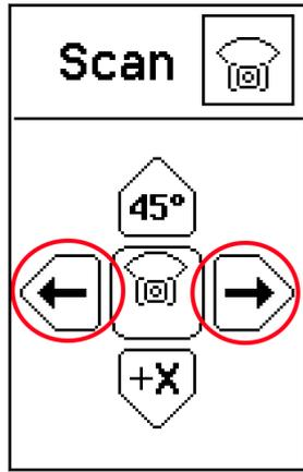
The scanning beam can be moved to the left or right side of the laser using the Scan 90 ° option.
