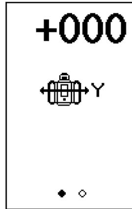
1. When the hour glass has disappeared, indicating that the Rugby has levelled, check both sides of the Y-axis.
