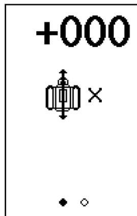
1. When the hour glass has disappeared, indicating that the Rugby has levelled, check both sides of the X-axis.
