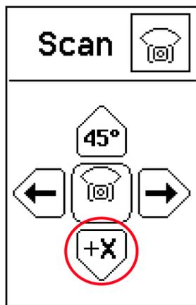
While in Scanning mode, the default direction of the scan is directly in the +X axis. Within the Scanning axis submenu, it is possible to redirect the scan to another axis.
