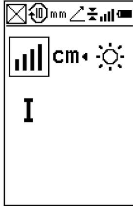
If there is no Rugby paired with the Combo a reduced menu screen is shown. This menu is limited to features that allow for the Combo to be used as a standalone receiver only.
