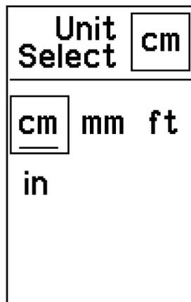
While a beam is being detected on the main screen, the digital read out displays the distance the beam is to the centre point on the Combo. Within the Unit settings menu, it is possible to select the units of the distance measurement:
