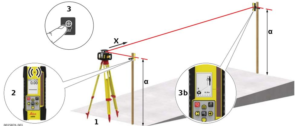
1. Set up the Rugby at the base of a slope with no grade dialled into the Rugby and with the X-axis pointing in the direction of the slope.
