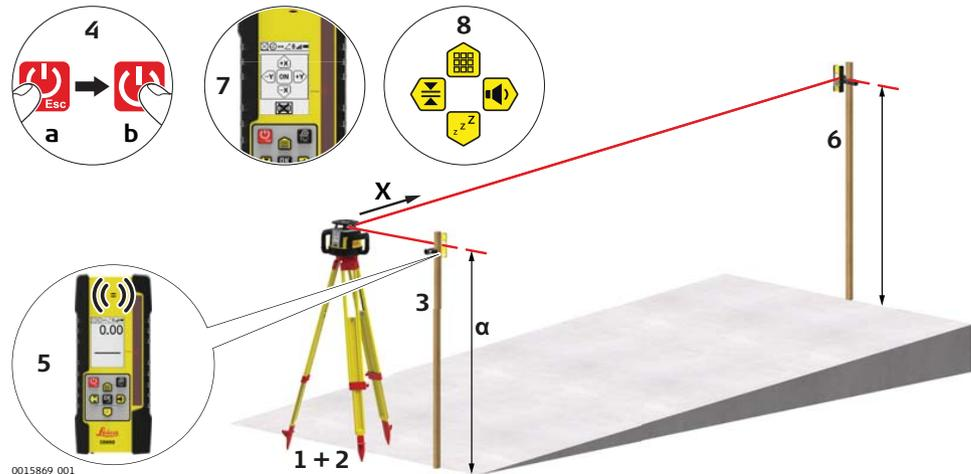
1. Set up the Rugby on a tripod.
