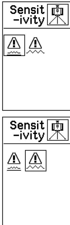
While levelling, the Rugby responds to disturbances, for example wind or vibrations, and stops the head rotation, if necessary. You can choose between two levels of sensitivity:
