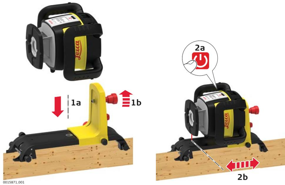
1. Mount the Rugby to the smart adapter and then the smart adapter to the batter board.
