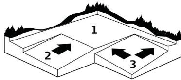
The Rugby CLH/CLA/CLI, depending on the configuration, is a dual grade laser. The laser produces an accurate plane of laser light for applications which require level (1), single slope (2) or dual slope (3).
